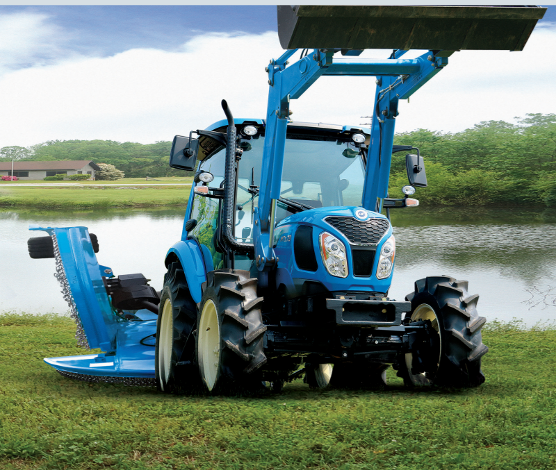
A wide field of vision The hood design combined with a large windshield and the sunroof provide a clear view with minimal obstructions.
