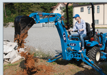
Powerful 6' backhoe The available sub-frame mounted backhoe can be quickly and easily attached or removed, unlike some competitive models without backhoe availability
