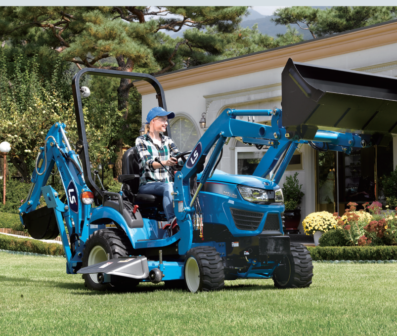
Excellent mower ground clearance The available mid-mount mower is easy to remove or attach and provide a full 6 inches of ground clearance
