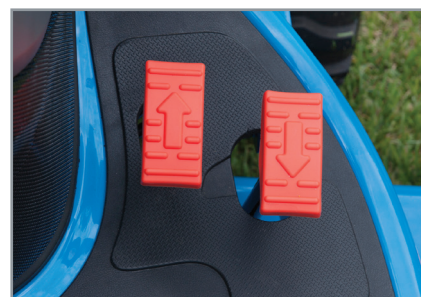
HST dual pedal Maximizes ease of use with effortless speed and directional changes
