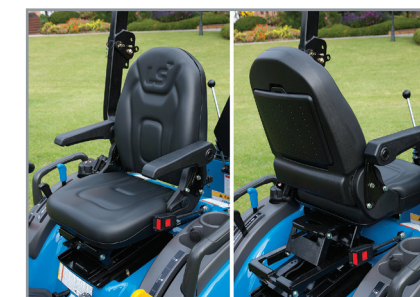
Comfortable High-Back Seat Supportive and comfortable seat reduces fatigue and reverses position for backhoe use
