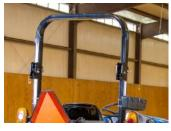
Standard Foldable ROPS **Enables Easy Adjustment** For Clearance
