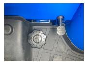
Mid-Mount Mower Height Adjustment Dial **Enables Precise Height** Control Of The Mid-Mount Mower, By A Simple Turn
