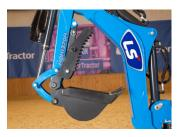
**Optional Thumb** Configuration Backhoe **Provides Added Functionality** To The Heavy-Duty Backhoe
