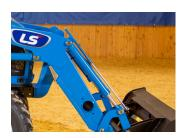
Loader Leveling Rod **Enables Operator To** Maintain Bucket Angle
