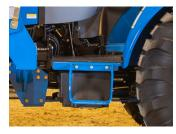
Accessibility Easy Access Platform Via Standard Step And Rubber Matted Surface
